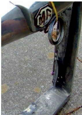
Tatty shell after removal of core. Cuts in side brass, stop water inlet fitting
