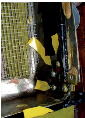
Bottom corner showing bolt heads, cut in side brass and new mounting bar
