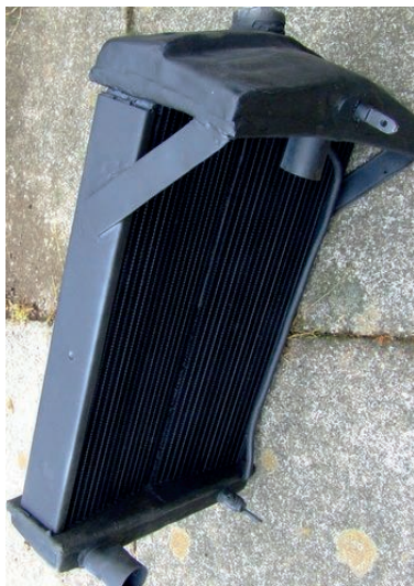
New radiator core. Note incorrectly angled water inlet.
