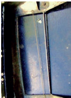
Repair to centre 'V', wire Tab. Note soldered top piece holding badge
