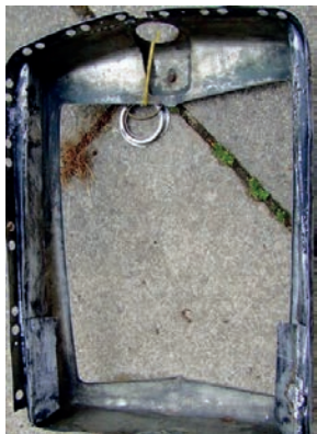
Tatty shell after removal of core. Cuts in side brass, stop water inlet fitting
